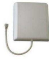
698-960/1710-2700MHz 7dBi Directional Panel Antenna
