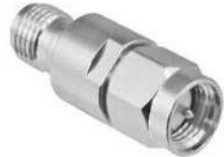
SMA Attenuator 2 Watts 3GHz 6dB
