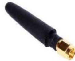
2.4 GHz 2 dBi Rubber Duck Antenna
