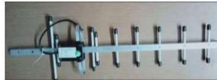
DIRECTIONAL YAGI ANTENNA - 12dBi
