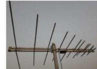
LOG PERIODIC DIPOLE ANTENNA 150-500MHz
