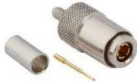
1.0/2.3 (SAA) MALE CRIMP CONNECTOR FOR RG 179 DOUBLE BRAIDED
