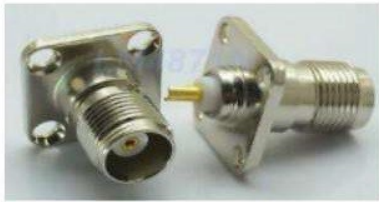
TNC Female 4H (17.5 Sq.) Flange Solder Pot
