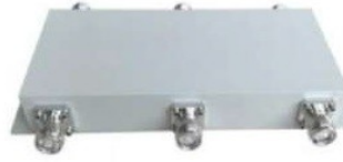
698 To 3800MHz 4.3-10 Female 3x3 Hybrid Combiner
